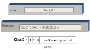
Fig 1: Data packet format for Multicast Routing
